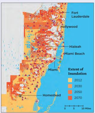
LEFT: In southeastern Florida, sea level rise drives a large increase in the amount of electricity infrastructure potentially exposed to flooding from a Category 3 hurricane over time. In total, 37 substations and two power-generating plants are at risk of inundation from a Category 3 hurricane today, compared with 119 substations and three power plants by 2070.
